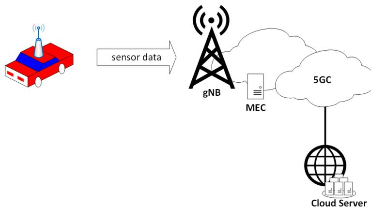
Figure 8. Overall architecture for *Vehicle Sourced HD Mapping*.
