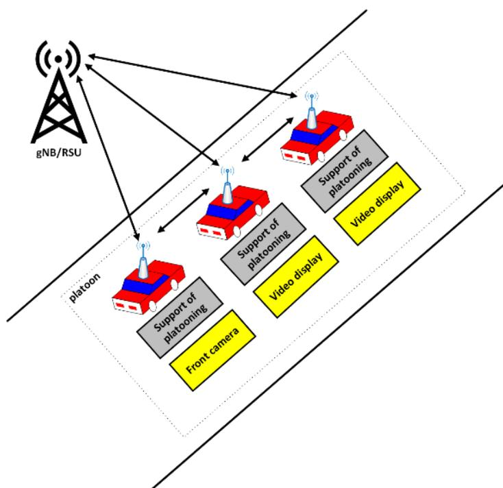
Figure 1. Architecture for *High bandwidth in-vehicle situational awareness and see-through for platooning*.
