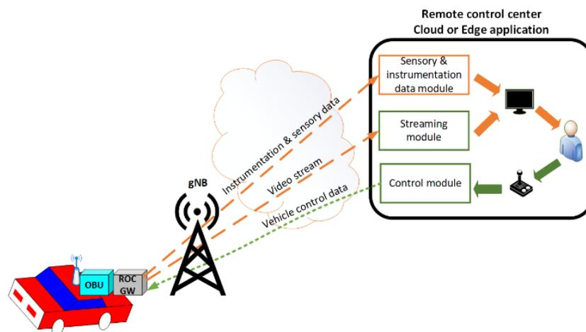
Figure 4. Overall architecture for TeSo.
