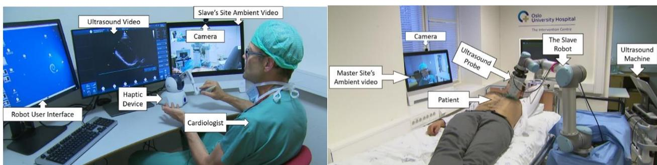
Figure 4. Robot-assisted remote ultrasound examination concept verification.
