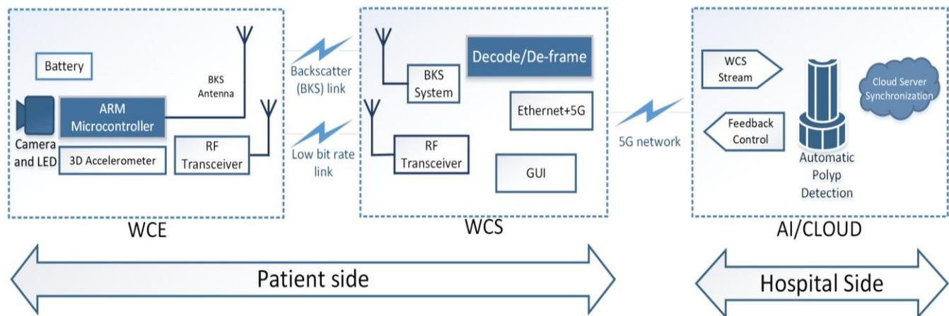
Figure 7. Wireless capsule endoscopy system.
