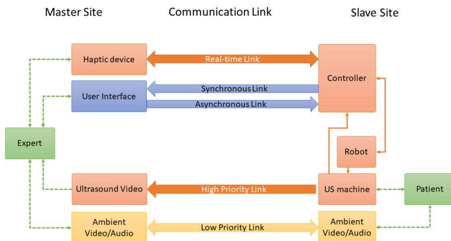
Figure 5. Robot-assisted remote ultrasound examination system architecture.
