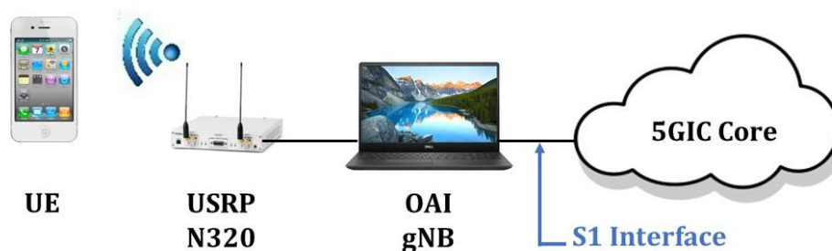
Figure 11. Experimental 5G setup #2; COST UE, OAI gNB and 5GIC CN
