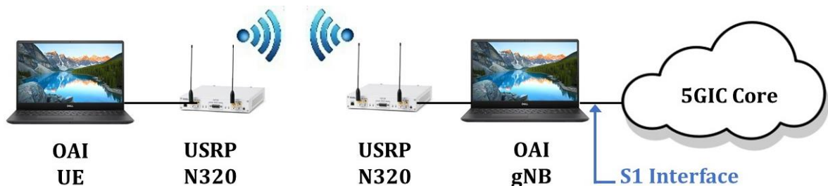
Figure 10. Experimental 5G setup #1; OAI RAN and 5GIC CN
